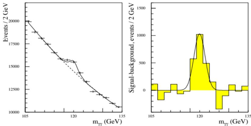
**Figure 19-4** Expected  $H \rightarrow \gamma\gamma$  signal for  $m_H = 120$  GeV and for an integrated luminosity of  $100 \text{ fb}^{-1}$ . The signal is shown on top of the irreducible background (left) and after subtraction of this background (right).
