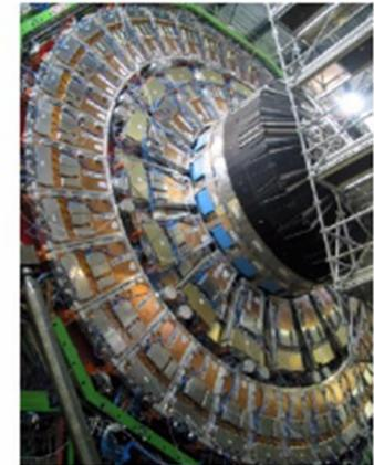
The ME1/3 CSC's now cover the RPC outer ring and hence complete the first Muon station on YE-1.
