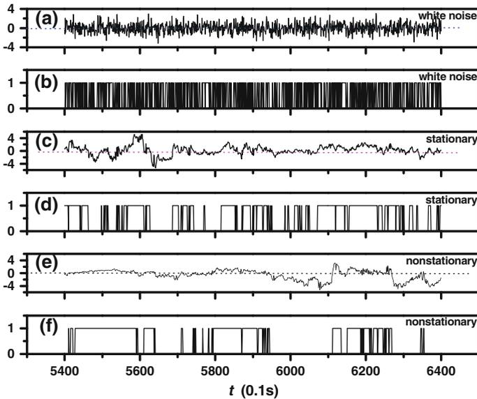
**Fig. 1** The normalized segments of **a** white noise, **c** stationary vertical velocity time series, **e** non-stationary vertical velocity time series and the TA results for white noise (**b**), stationary series (**d**) and non-stationary series (**f**). Since the TA only takes values of 1 or zero, no amplitude variations are considered
