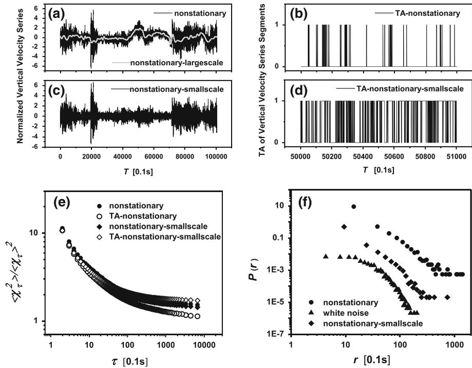
**Fig. 7** Extracting large-scale fluctuations from the original non-stationary vertical velocity time series (a), we obtain small-scale fluctuations (c); b, d are segments of the TA results of (a) and (c). The intermittency exponents for the original time series and their small-scale fluctuations are shown in (e); f shows the distributions of the inter-pulse periods
